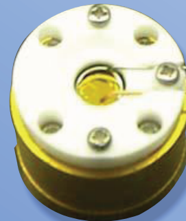
Liquidcell with contacted sample and reference electrodes
